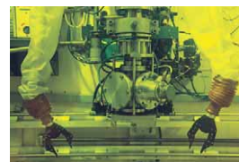
Vertical beam line for irradiation of solid and gas targets.
