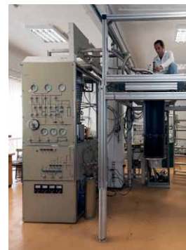
The dilution refrigerator for experiments in mK temperature range
