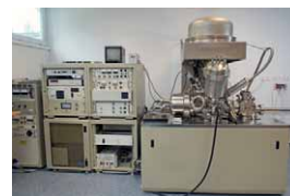
The VG ESCASCOPE electron spectrometer for XPS, monochromated XPS and laterally resolved XPS measurements.
