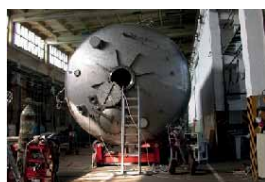
Vacuum leak testing of large-scale industrial facilities (fermentation tank). VTMT Ltd, spin-off company of Atomki.
