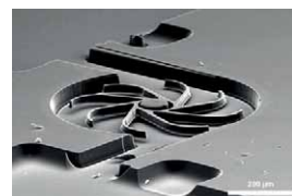
Microturbine made by PBW and subsequent selective porous Si etching in collaboration between MTA Atomki and MTA TTK MFA.
