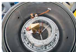
Experimental setup with the electrostatic spectrometer for molecule fragmentation experiments.
