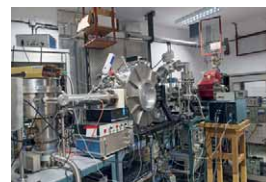
Time-of-flight electron spectrometer for studies of ion-atom collisions.
