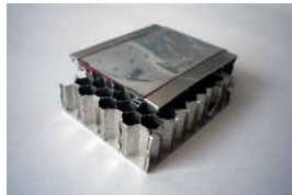
This multilayer plate was developed for thermal protection of Smart-1, but the surface cracked during the radiation hardness tests performed in Atomki
