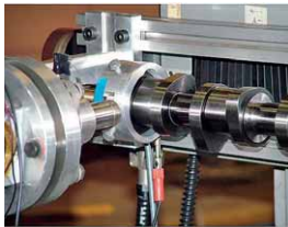
Automobile camshaft irradiation for wear measurement by using TLA (Thin Layer Activation)
