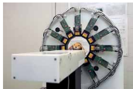
The MiniPET-3: small animal PET scanner for preclinical studies (for more details see page 43).
