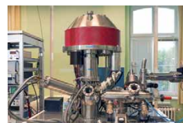
The high-energy home-built ESA-31 electron spectrometer for XPS, XAES, HAXPES, REELS and EPES measurements.
