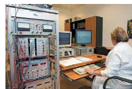
Gas proportional counter system for high-precision ^{14}\text{C} dating + pre treatment unit (Atomki).
