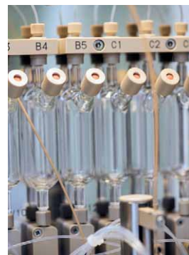
Valve system of the equipment for radiopharmaceutical production.
