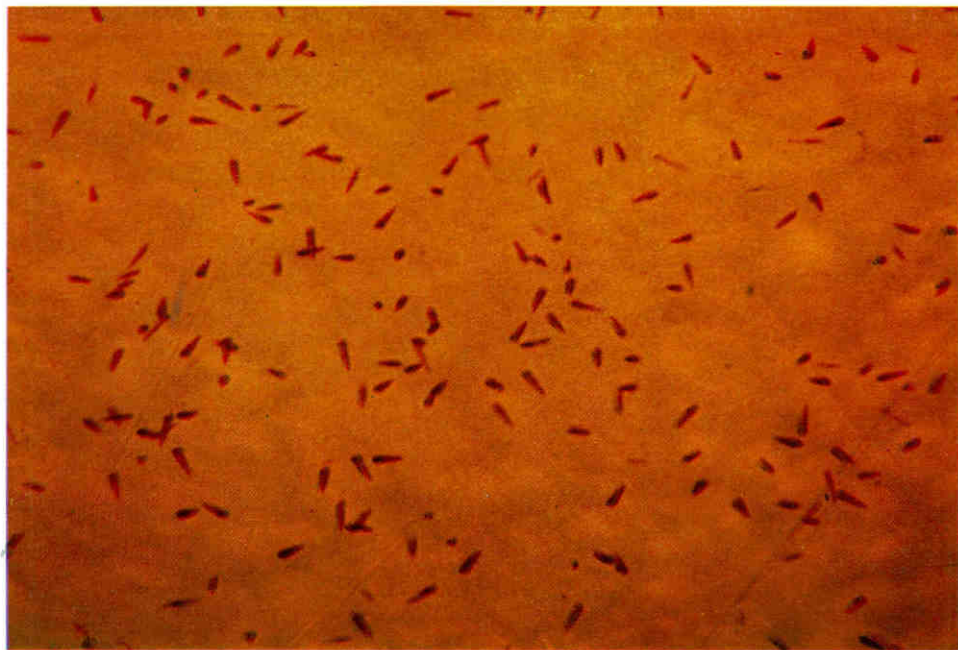
Tracks of alpha particles in solid state track detectors. The tracks have been developed by a new technique worked out in ATOMKI
