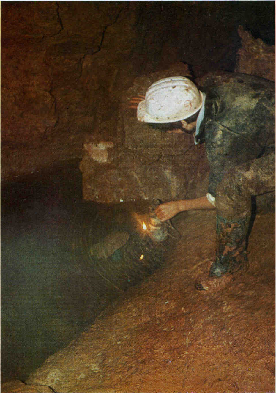
Measuring the radon content of air in a cave by solid state track detectors
